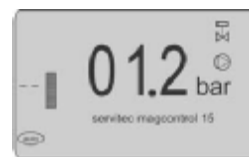
Display automatic operation with interval deaeration --
